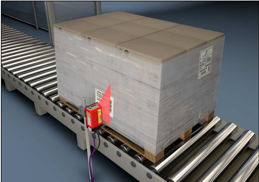
Figure 4.10: Deflection principle for the line scanner
