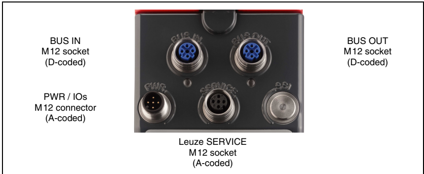
Figure 7.1: Connections of the AMS 348 i
