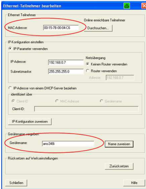
Figure 9.10: Linking of the device name to the MAC ID of the participant
