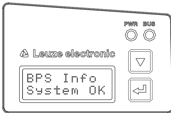
Figure 10.2: Example: Device status/error status information on the display
