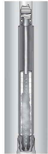
Vapor quenches arc at first current zero
