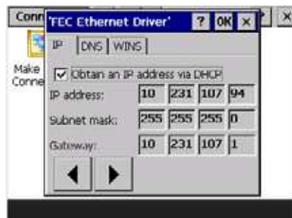
Figure 36:WinCE – Ethernet/IP settings
