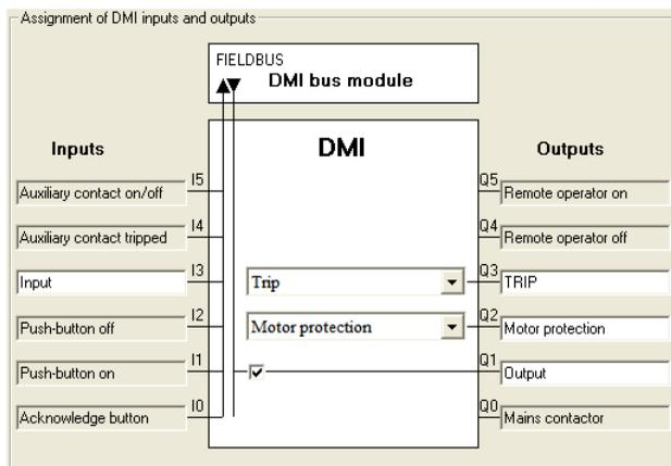
Figure 47: Example assignment of DMI inputs and outputs
