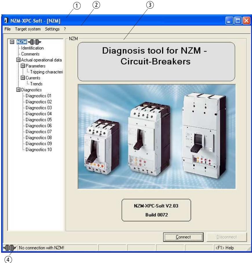
Figure 4: User interface with start-up screen in NZM mode
