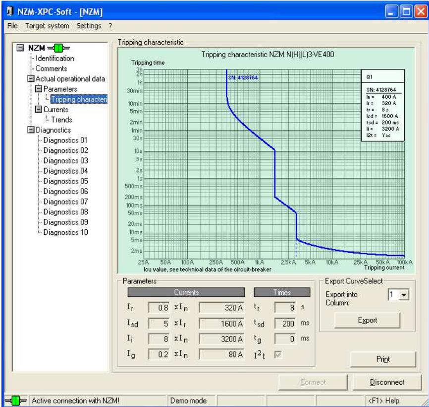
Figure 20: Tripping characteristics of the NZM
