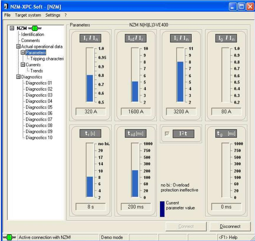
Figure 19: Actual parameters for the connected NZM
