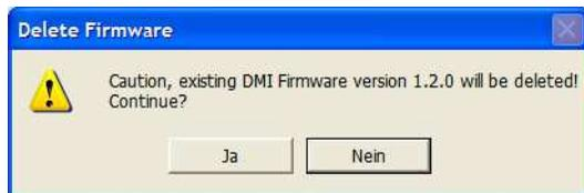
Figure 56: Warning message before the firmware is deleted
