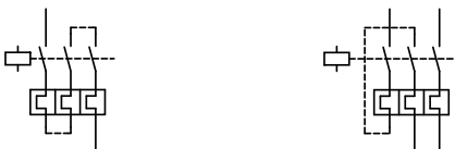
Figure 4: Wiring of the motor-protective circuit-breaker for the protection of AC or DC motors (bimetallic release switched in series)
