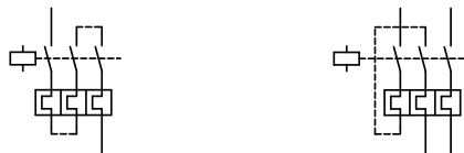
Figure 16: Wiring the PKE motor-protective circuit-breaker for protecting AC motors (series connection of the overload releases)
