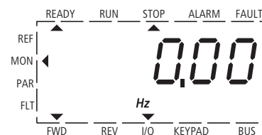
Figure 101:Operational data indicator (operational)
