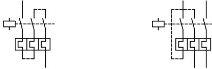
Figure 6: Wiring of the overload relay for the protection of AC or DC motors (bimetallic release switched in series)
