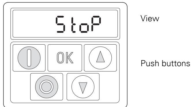
Figure 1: Operating unit view
