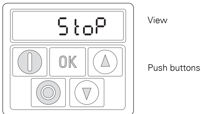
Figure 1: Operating unit view
