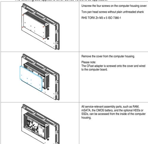
Abb. 7 Opening the device
