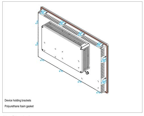
Abb. 3 Fixing and sealing
