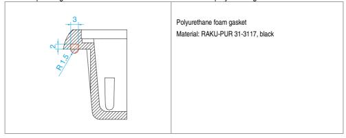
Abb. 4 Polyurethane foam gasket
