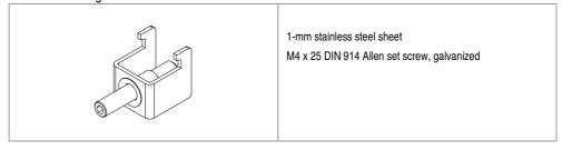
Abb. 5 Device holding bracket
