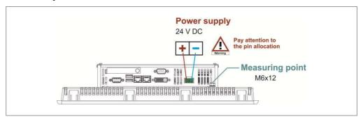
Abb. 6 Connecting the 24 VDC supply voltage
