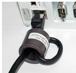
Abb. 40 Ethernet cable with double loop through ferrite core
