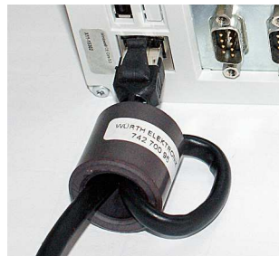
Abb. 34 Ethernet cable with double loop through ferrite core
