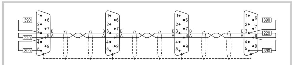
Abb. 22 Bus segment with four bus stations
