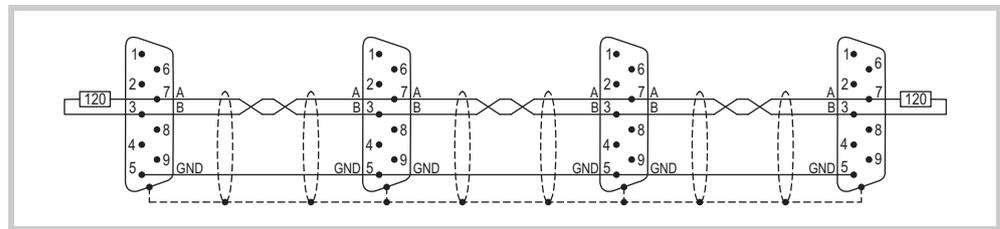
Abb. 24 Bus segment with four bus stations
