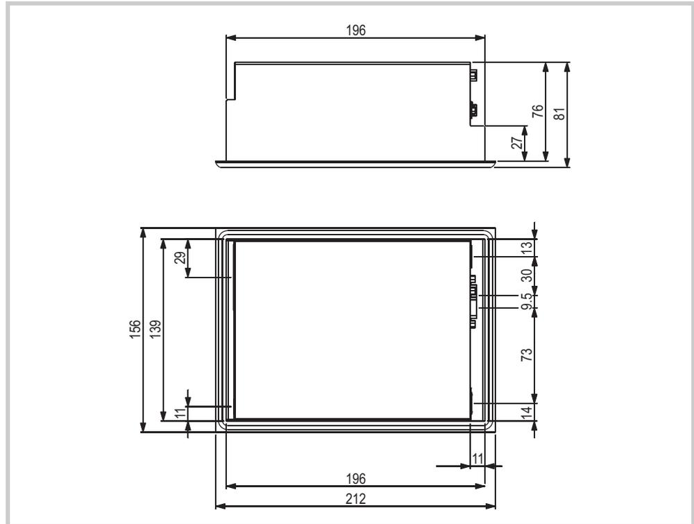
Abb. 33 Mechanical dimensions of the SKS devices in mm
