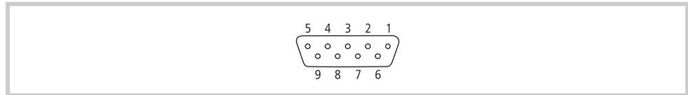
Abb. 21 Profibus interface (9-pin, D-Sub, female, UNC)
