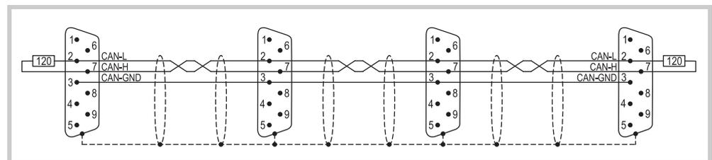
Abb. 20 Bus segment with four bus stations
