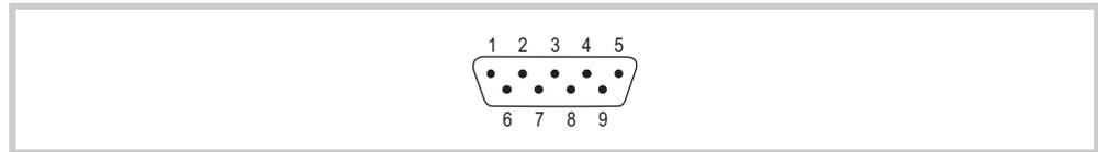
Abb. 19 CAN interface (9-pin, D-Sub, male, UNC)
