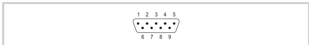
Abb. 16 RS232 interface (9-pin, D-Sub, male, UNC)
