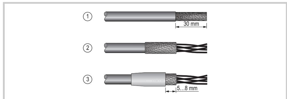
Abb. 12 Connecting the cable shield
