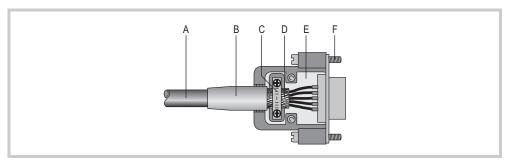
Abb. 13 Cable prepared with D-Sub connector
