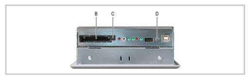
Abb. 6 Operating elements on the service side (CF slot cover removed)
