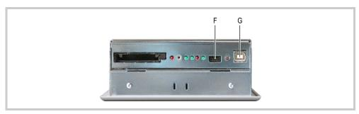
Abb. 11 Interfaces on the service side of the BAS, CAN and MPI devices (figure shows service side of BAS, CAN and MPI devices)
