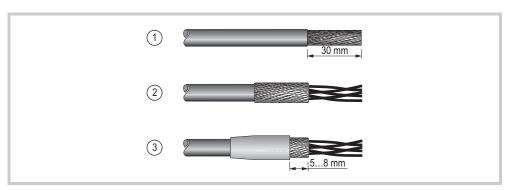
Abb. 12 Connecting the cable shield
