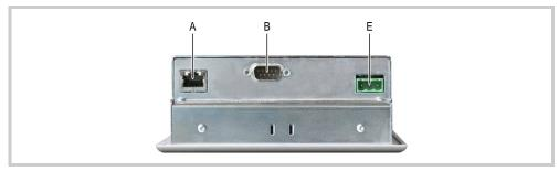
Abb. 9 Interfaces on the connector side of the BAS, CAN and MPI devices (figure shows CAN device)
