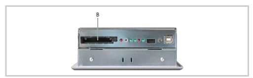
Abb. 31 Service side of the device (CF slot cover removed)
