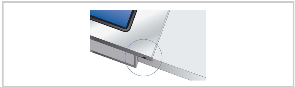
Abb. 43 Device front plate is flush mounted
