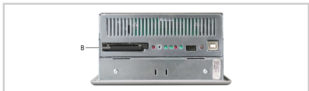
Abb. 46 Service side of the device (CF slot cover removed)
