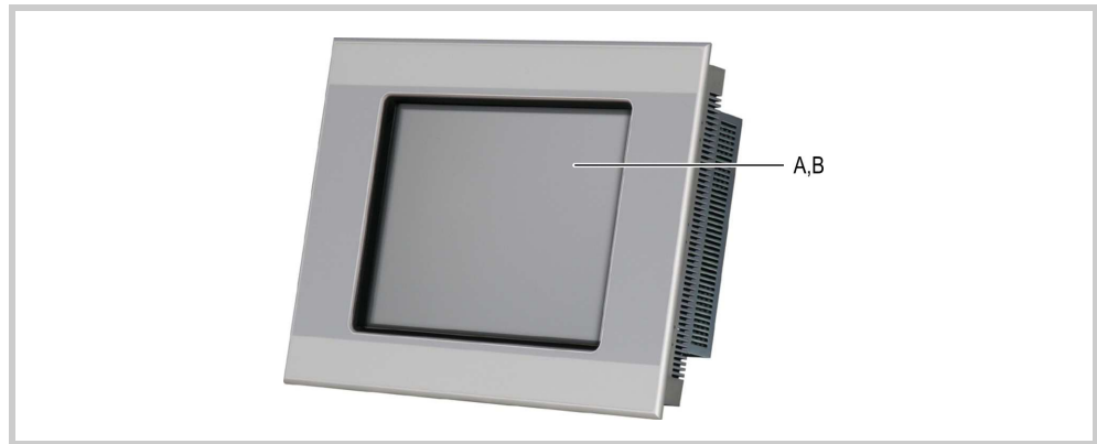
Abb. 5 Operating and indication elements on the front (figure shows device with infra-red touch)
