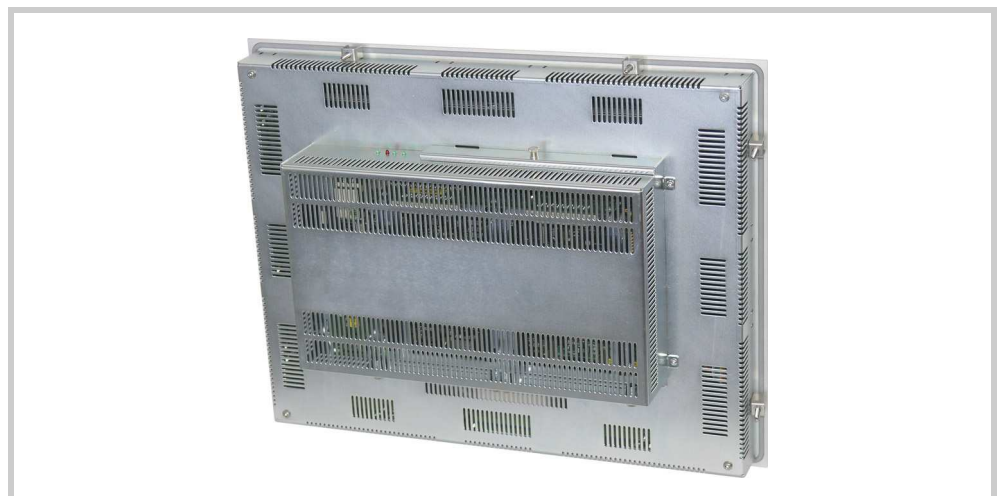
Abb. 43 15" devices with eight retaining brackets (do not meet IP65 requirements)
