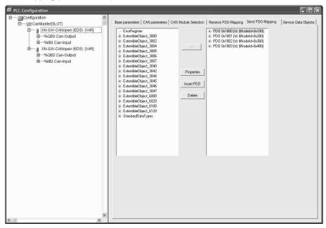
The tabs **Receive PDO mapping** and **Send PDO mapping** in the configuration dialog allow the "mapping" of the module described in the EDS file to be changed.
