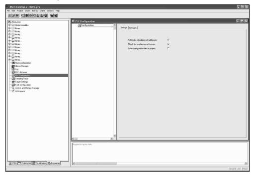
The PLC configuration is displayed in the editor in tree structure and can be edited using menu commands and dialogs. The configuration contains input and/or output elements and also management elements which themselves also have subelements (for example, CAN, PROFIBUS).
