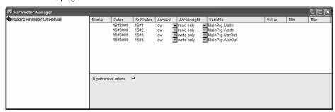
In order to be able to open the Parameter Manager, it must be activated and defined with correct index/subindex ranges in the map 'Network functionality' of the target settings.
