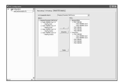
The **Default-PDO-Mapping** tab allows the entries which are defined in the Parameter Manager to be assigned/modified to the "Mapping" of the CAN-Device.
