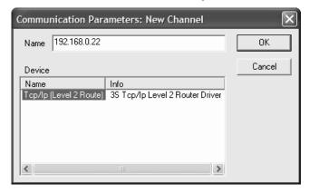
The name used for the last entered channel is automatically proposed in the **Name** entry field. You can edit here the channel names. The channel names are solely for information, uniqueness is not mandatory but is recommended.
