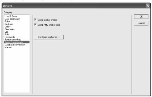
The **Configure symbol file** button is used to define from which objects the variables are exported into the symbol file.
