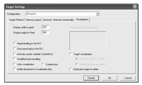
Depending on the used PLC target system, Target visualization and Web visualization are supported. Appropriately information is given in the table below.
