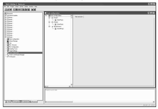
Each task can be assigned a sequence by programs, which are to be executed by the call of the task. The task priority and task condition specify, in which timing sequence the tasks are to be processed. A PLC program can consist of several tasks of the same or a different priority, which are processed cyclically in parameterized time intervals or when particular events occur.
