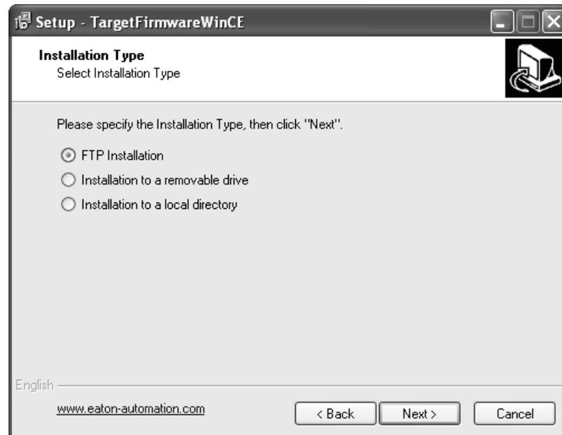
**FTP Installation** : The installation of the directories **PicRts** and **PicPrg** is made by FTP.
