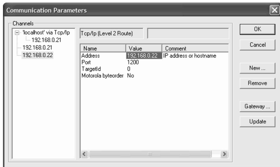
The parameters for a channel already known by the gateway server can no longer be edited in the configuration dialog. The parameter fields appear grey. You can, however, delete the connection as long as it is not active.
