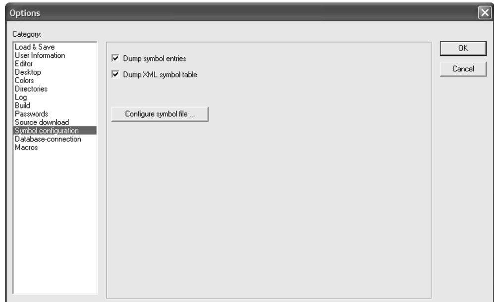
The **Configure symbol file** button is used to define from which objects the variables are exported into the symbol file.
