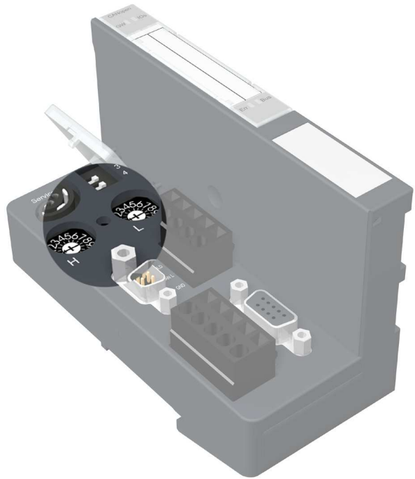
Figure 17: Rotary hex encoding switch for addressing setting of the XN-GW-CANopen
