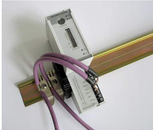
Figure 22: Shielding the bus cable via shielding brackets on the mounting rail
