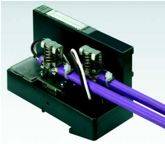
Figure 13: Shield connection (gateway)
