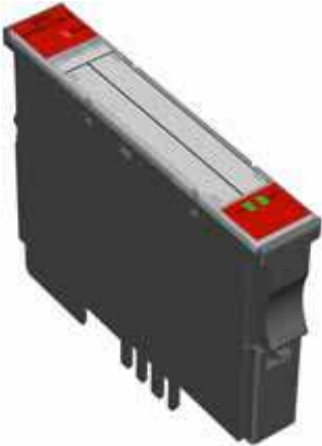
Figure 80: Digitale output module, 2 digital outputs, 24 V DC, 0.5 A, positive switching
