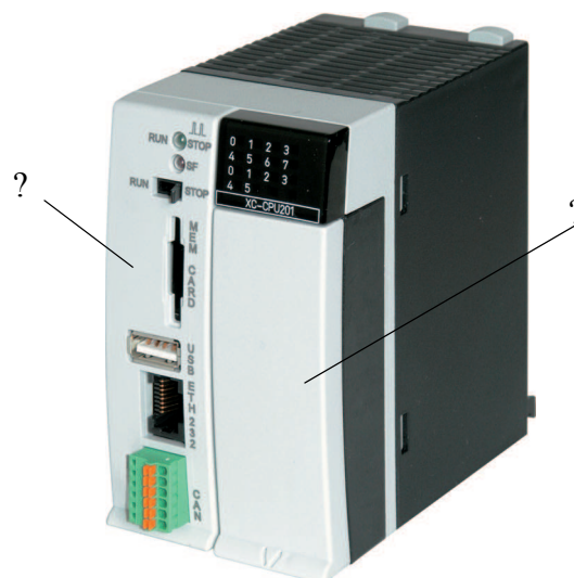
Figure 2: XC-CPU201 – a CPU of the XC200 series
