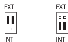
Figure 82: Connecting the external supply voltage with jumpers
