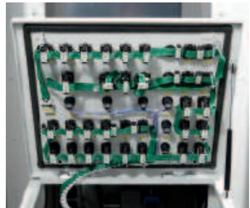
easy800 with SmartWire-DT controls control circuit devices – easily, quickly and efficiently.
