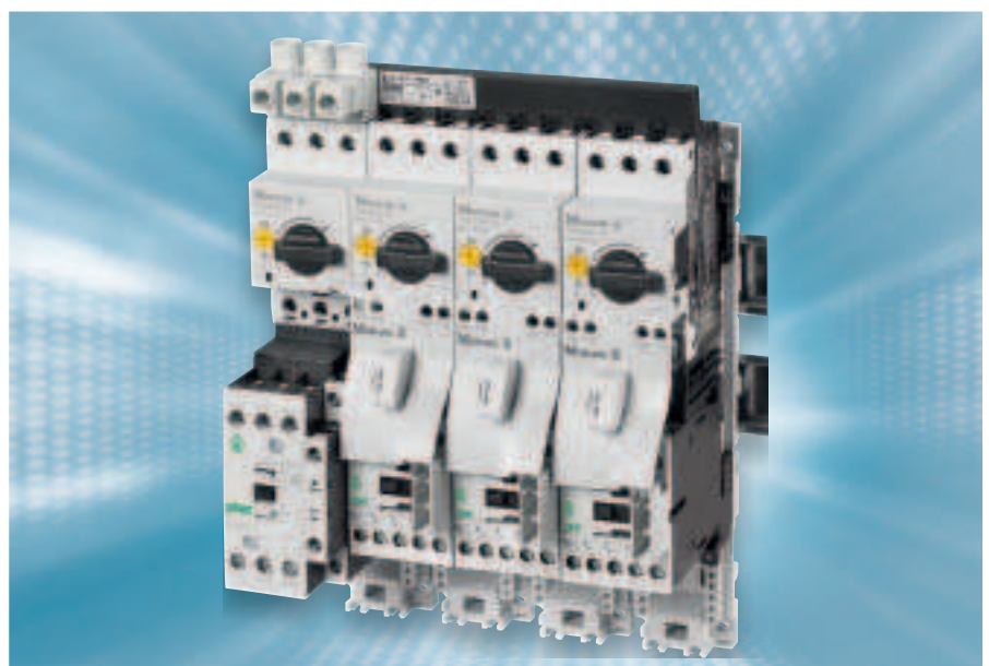
Figure 24: Example of UL 508 Type F Combination Starter combined from manually operated UL 508 Type E devices and contactors. The combinations have to be listed in switchgear manufacturer's Approvals files.
