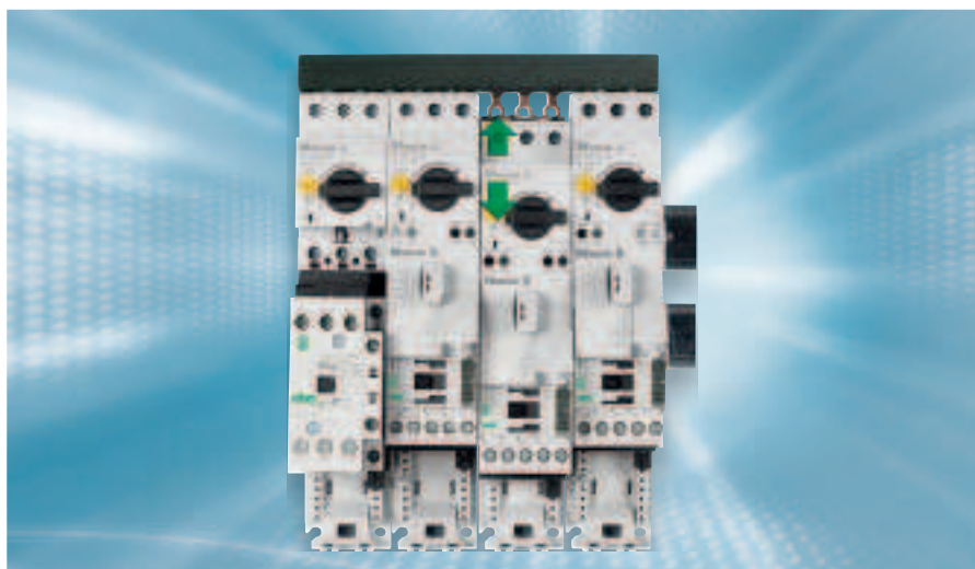
Figure 14: Mounting rail adapters have two independently movable mounting rails that make insertion and removal of individual components easy without having to disassemble the three-phase commoning link.
