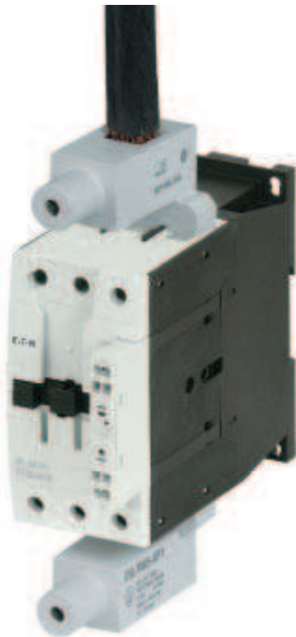
Photo 9: The paralleling bridge allows the AC-1 "General Purpose" 3 phase current rating of the contactor to be increased by a factor 2.5 times its value. This accessory is especially useful when switching single phase resistive loads (such as heaters). It permits the use of smaller, and more economical, contactors to handle the load.
