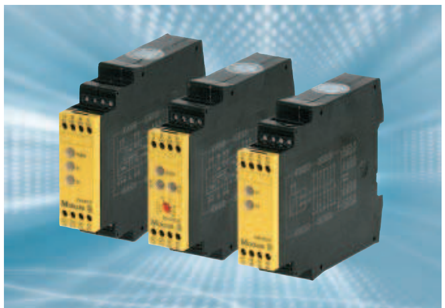
Figure 7: The safety relay ESR 4-.. in a 22.5 mm wide enclosure is available from Moeller as a processing alternative for standardised safety circuits. Space is saved in comparison to the parallel connection of several contactor relays and the wiring and testing expense is reduced.
