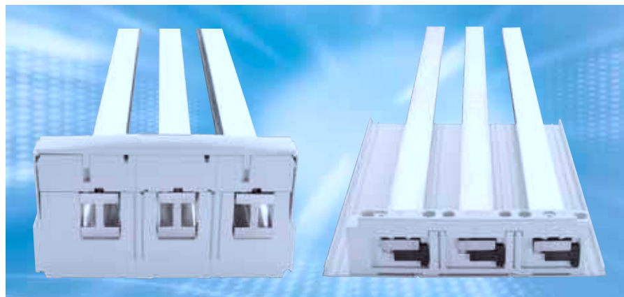
Photo 5: Busbar holders with UL/CSA certification for world-wide applications. Use of an additional bottom plate is necessary in North America in order to establish the appropriate electrical clearances between the bus and the mounting plate.
