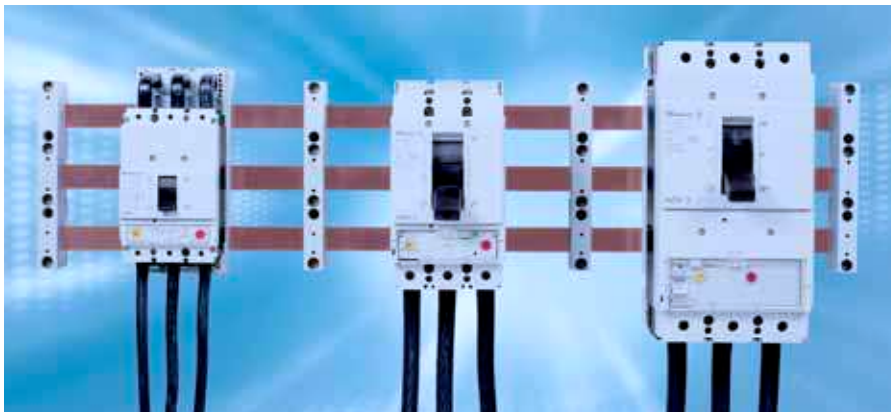
Photo 3: It has become possible in the meantime to design adapters which allow mounting of circuit breakers or molded case switches, rated up to 550 A and used in incoming or outgoing circuits, directly onto the busbar system. The actuation possibilities for the switches can also be varied, from manual means to remote switching via an electrical motor operator, or even through a flex cable and side handle accessory typical of North American installations.
