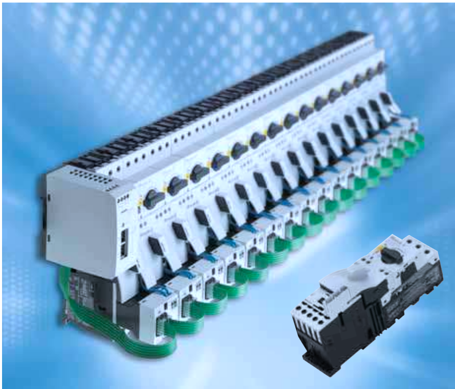
Photo 1: The latest networking system Smart Wire from Moeller is used primarily to replace conventional control circuit wiring in motor starters, such as actuation of contactor coil and status indication of contactor energization. The connection of individually mounted starter units, which can also be mounted on busbar systems, is established via pre-assembled flat ribbon cable connectors with suitable end plugs.
