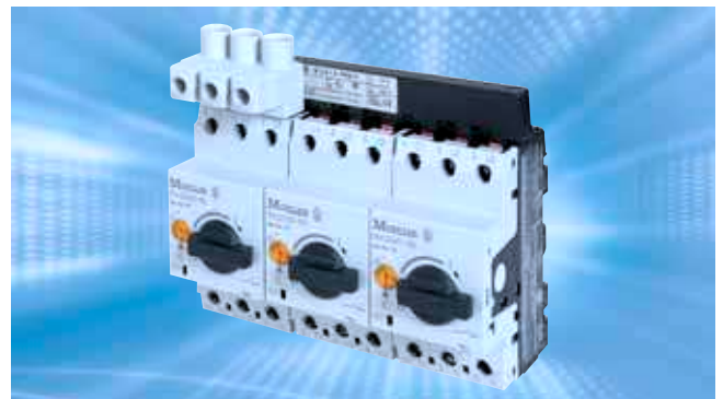
Photo 12: 3 UL 508 Type E- Motorstarters (Manual Type E Self-Protected Combination Motor Controller), shown here as a small grouping with bus link connectors for use e.g. in a decentralized automation process. Of particular interest is the large spacing terminal block BK25...-E, which in this particular array would only need to be used once to provide the larger electrical clearances for the incoming supply. This terminal must be provided on each individually equipped motor starter adapter destined for export to North America.
