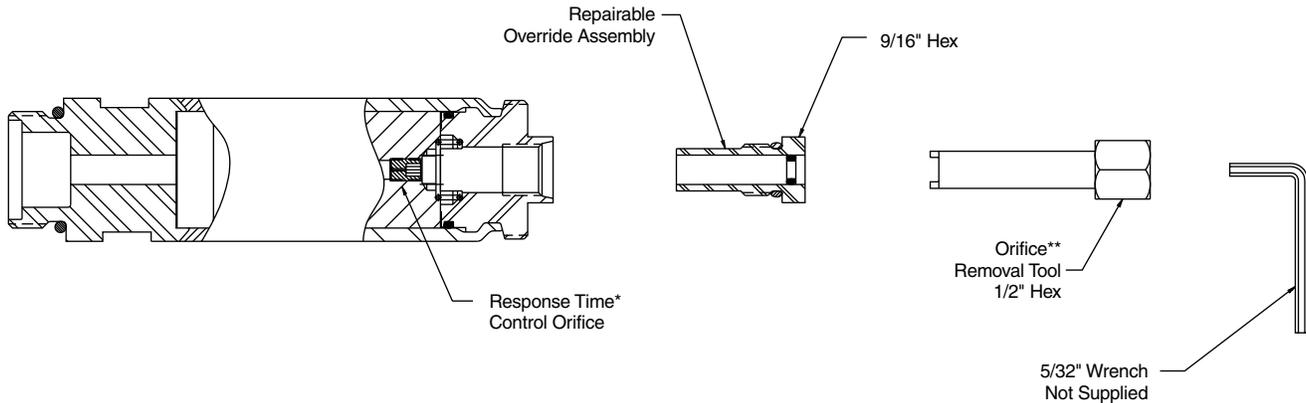
\*\* Orifice Removal Tool with Kit Part Number 1301661
