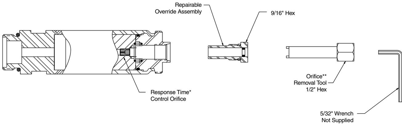
\*\* Orifice Removal Tool with Kit Part Number 1301661
