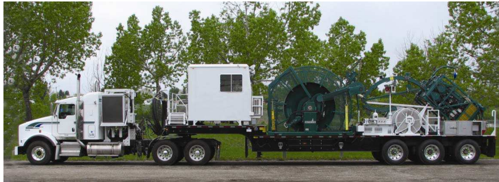
Coiled Tubing Unit
