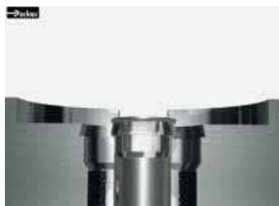
The tube end is released and can be taken out of the machine
