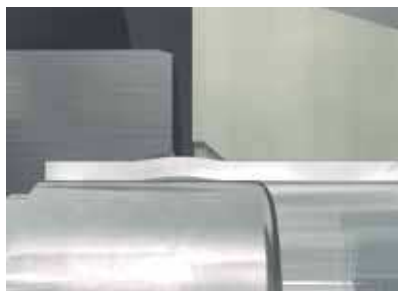
While moving, the pin is continuously forming the tube wall and compressing the material
