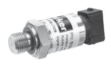
Weight 0.06 kg -40 °C to 125 °C Operating temperature Storage temperature -40 °C to 140 °C Pressure range 0 - 35 bar SP035 0 - 500 bar SP500 Over pressure Max 100 bar SP035 Max 1050 bar SP500 Burst pressure SP035 Min 150 bar SP500 Min 1500 bar Total error (-40°C to 105°C)1) Max 4.0 % FS Total error (40°C to 80°C)1) Max 1.0 % FS
