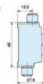
swivel elbow push-in connector 4 mm OD tube
