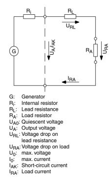
The **output characteristic** diagram at right shows the generator characteristic and the resistance line of the valve. The difference between the  $U_{RA}$  and the actual output voltage  $U_A$  meets the maximum voltage drop across the cable. From that, the maximum cable length and resistance can be calculated.
