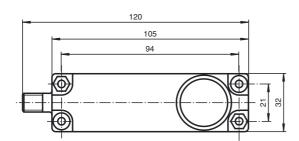
Bore hole and countersinking for screws/hexagon M4
