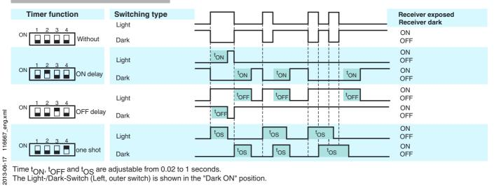
Time  $t_{ON}$ ,  $t_{OFF}$  and  $t_{OS}$  are adjustable from 0.02 to 1 seconds. The Light-/Dark-Switch (Left, outer switch) is shown in the "Dark ON" position.
