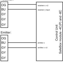
Design with terminal compartment Receiver:
