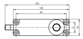
Bore hole and countersinking for screws/hexagon M4
