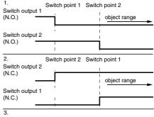
Switch point 1 ->  $\infty$ : Switch output 1, (N.C.) Detection of object presence Switch point 2 ->  $\infty$ : Switch output 2, (N.O.) Detection of object presence
