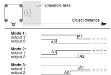
A1  $\longrightarrow \infty$ , A2  $\longrightarrow \infty$ : Object presence detection. Both outputs operate according to the selected mode, if an object is located within the detection range.
