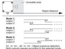
A1  $\rightarrow \infty$ , A2  $\rightarrow \infty$ : Object presence detection. Both outputs operate according to the selected mode, if an object is located within the detection range.
