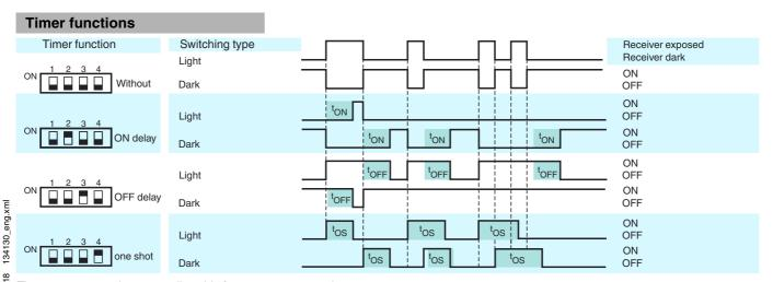
Time  $t_{ON}$ ,  $t_{OFF}$  and  $t_{OS}$  are adjustable from 0.1 to 10 seconds. The Light-/Dark-Switch (Left, outer switch) is shown in the "Dark ON" position.
