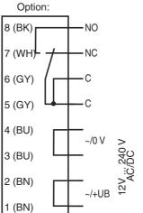
The relay-functions "NC" and "NO" bear on the switching mode "Dark-ON".
