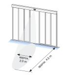
Installation height 2200 mm / angle of detection field 30°
